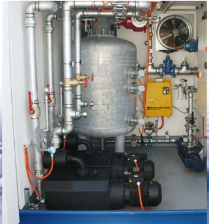
HVE-container with blowers, liquid separator and control panel
