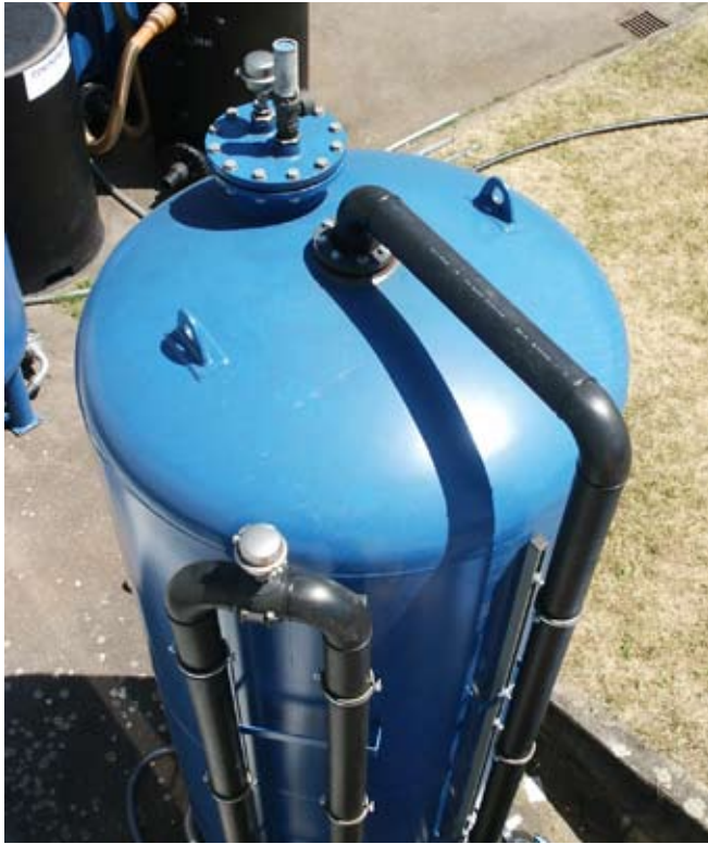
Ports (inspection, cleaning) at the back of the Shallow Tray stripper
